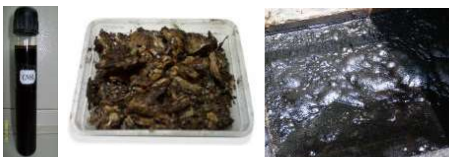
Fig. 2: CNSL, cashew shell cake and CNSL contaminated waste water from cashew processing unit
