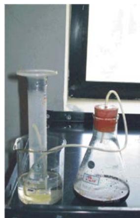
Fig. 3: Water displacement study to test methane production by E.Coli strain
