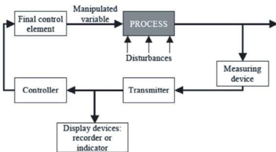
Fig. 1: Typical control system components
