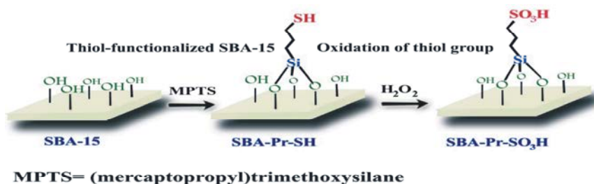
Fig. 2: Schematic illustration for the preparation of SBA-Pr-SO 3 H.
