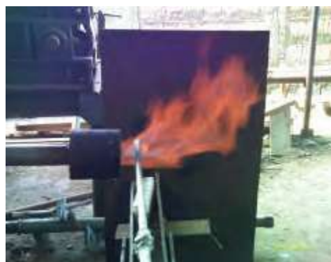
Fig. 2: Flame of gas combustion
