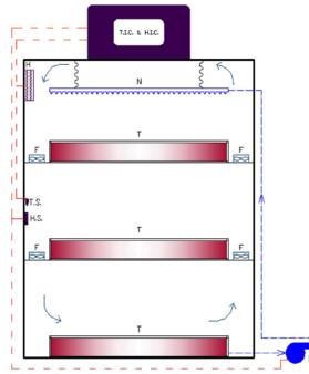
Fig. 1: Schematic diagram of the tray bioreactor set up;
