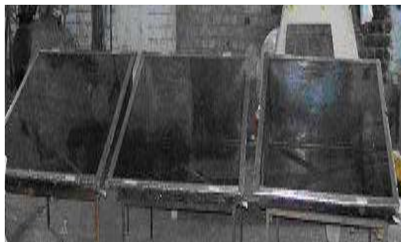
Fig. 1: Experimental Set up of Solar stills
