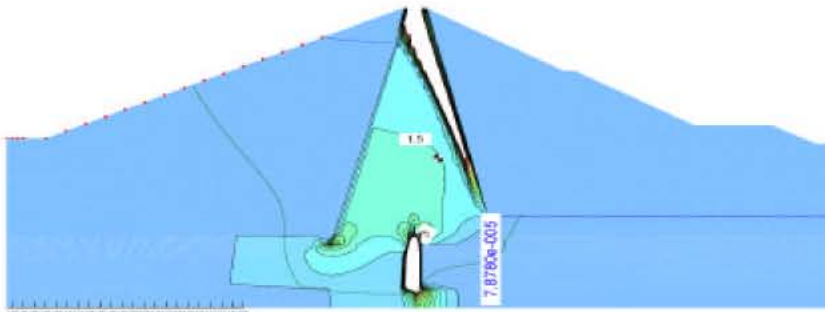
Fig. 7: Model with up saturation and semi saturation for core and downstream
