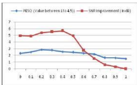
Fig. 3: Plot of PESQ level and SNR improvement (y-axis) versus reduction factor K_{red} (x-axis) for a given speech signal
