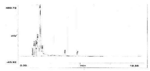
Fig. 1: HPLC Chromatograph of Soya Oil Methyl Ester
