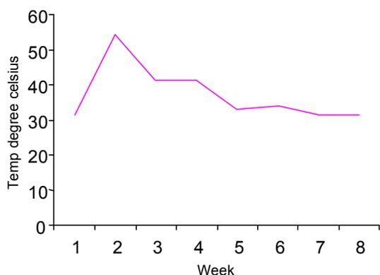
Fig. 4: Temperature changes during biodung composting
