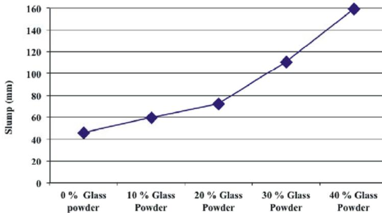
Fig. 1: Slump values of concretes with varying amounts of glass powder
