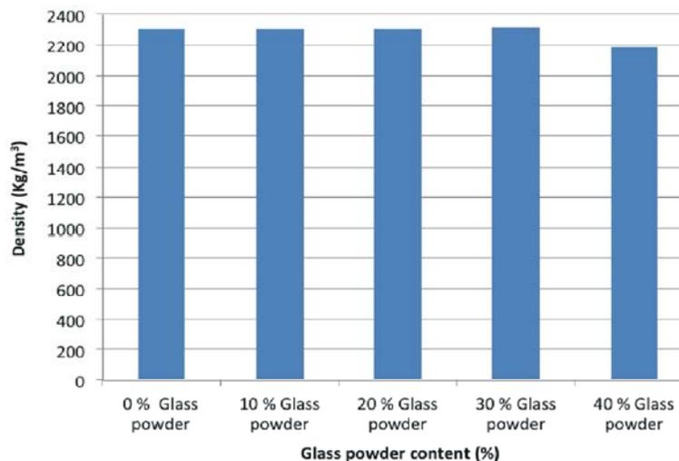
Fig. 2: Density of concretes with varying amounts of glass powder
