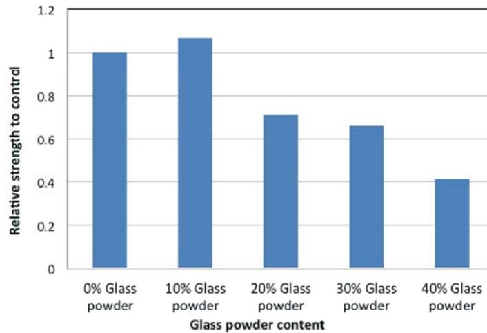
Fig. 4: Relative compressive strength to the control at 28 days of curing of concrete with varying amounts of glass powder.
