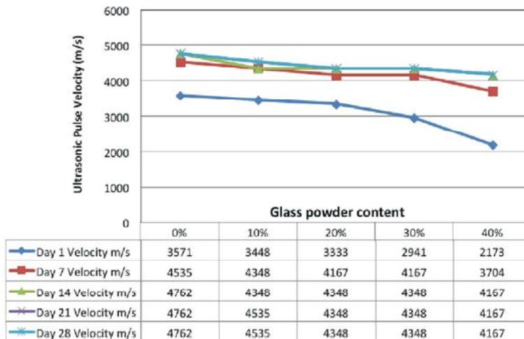
Fig. 5: Ultrasonic pulse velocity for concretes containing varying amount of ground glass at different ages of curing.
