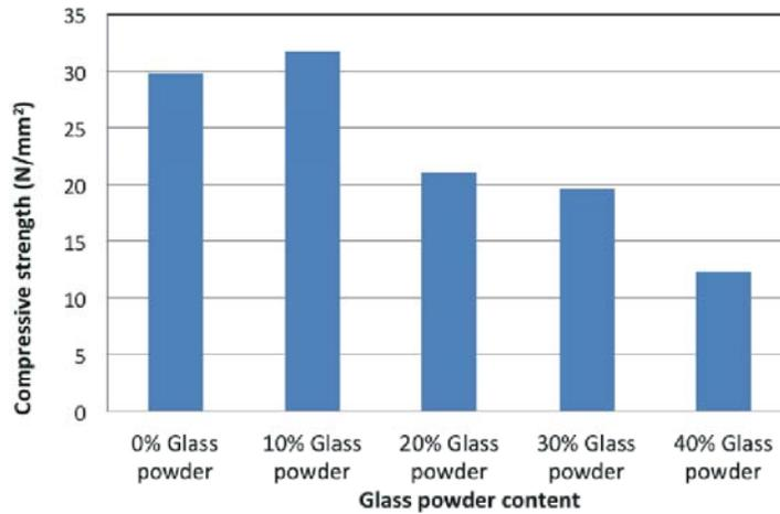
Fig. 3: Compressive strength of concretes with varying amounts of ground glass at 28 days of curing
