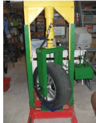
Fig. 2: Tire contact area measurement apparatus
