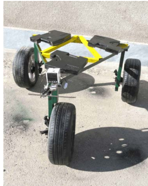
Fig. 1: The tire rolling resistance test apparatus, linkages, weights, load cell and data logger
