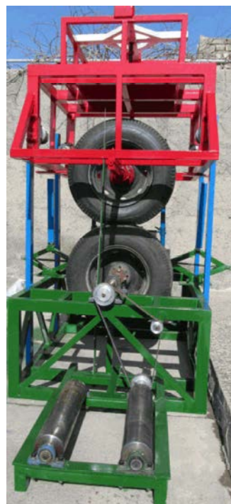
Fig. 3: Tire contact length measurement apparatus
