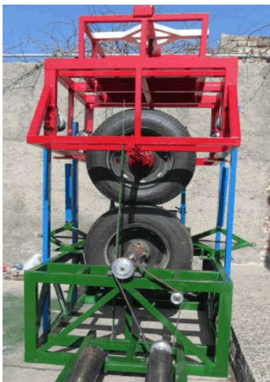
Fig 2: Tire deflection test apparatus
