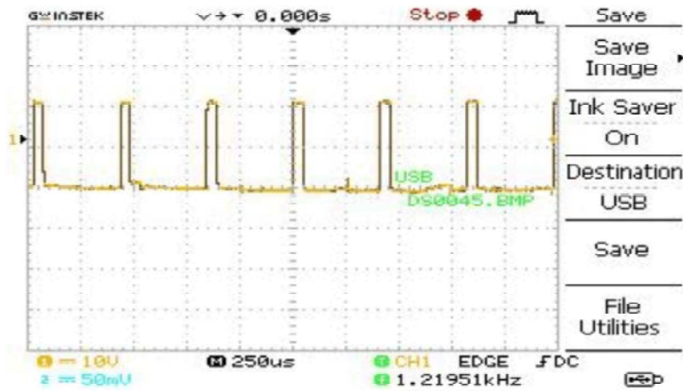
Fig. 15: Gate Pulse to Rectifier Switch S2
