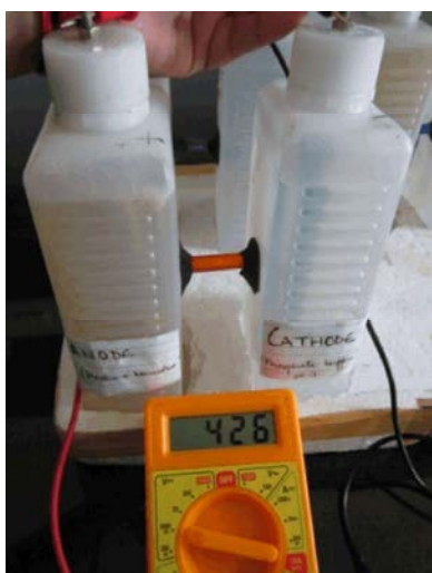
Fig. 2: The MFC constructed in the lab attached with a multimeter
